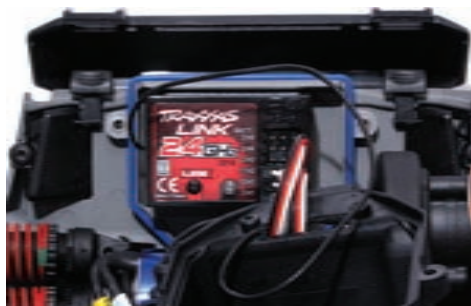
2.4 GHz as standard, note the twin channel 1 ports...for twin steering servos
