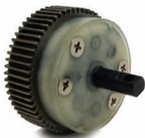
Above: Not 100% sealed, but pack it with grease not oil and you're onto a winner
