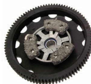
Above: Three shoes on my slipper... back it off about a turn to protect the diff and driveline!
