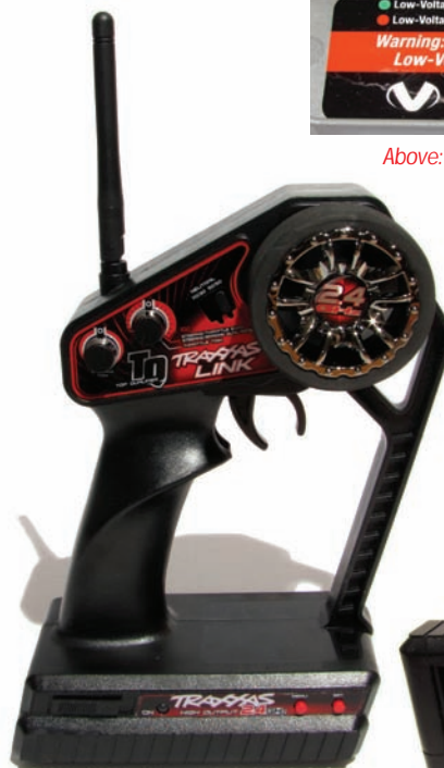
Left and below: The 2.4 GHz TQ Tx has features you would expect of a much higher priced spec item Dual rate, 20 model memory and end point adjustment to name but three
