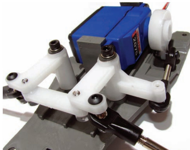
Above: A waterproof 2027 Digital servo takes care of the steering, well protected by a large servo saver
