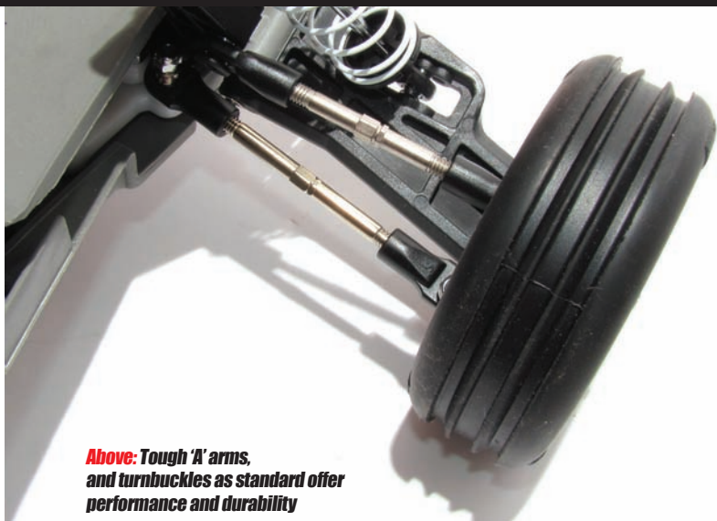
Above: The front axles spin on shielded bearings, and as ever all components are 'Traxxas Tough'
