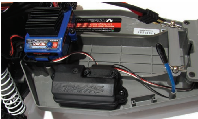
Above: Waterproof receiver box and potted waterproof VXL ESC allow you to run where others fear too!
