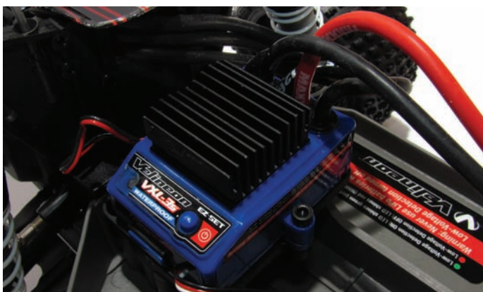
Above: The Velineon VXL-3S ESC offers both sensorless and sensed operation, brushed or brushless motor configurations...
