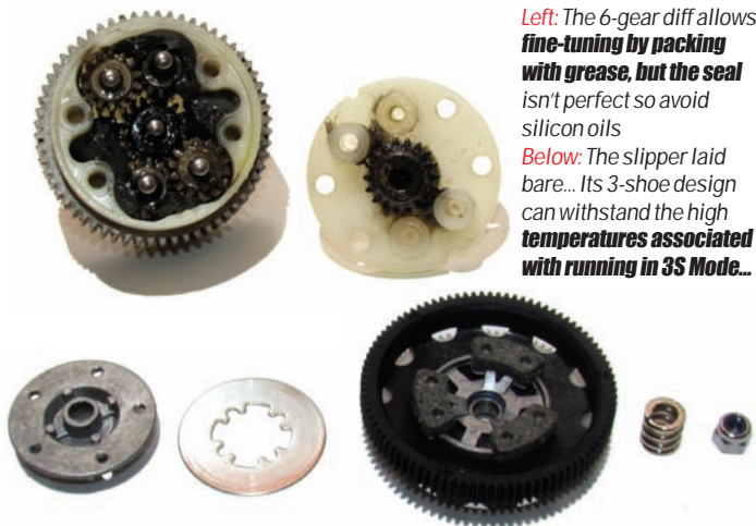
Above: The 3-shoe slipper is a Revo-spec item, meaning it can handle anything thrown at it
