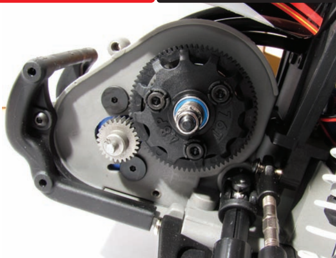
Above: The 3-shoe slipper is a Revo-spec item, meaning it can handle anything thrown at it
