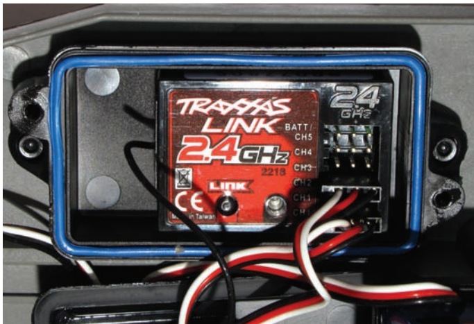
Above: The Link system means that the Tx will remember the settings and model memory for up to 20 receivers without you doing a thing!
