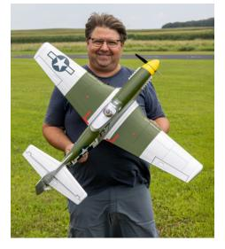
for experienced pilots. The BNF Basic version is equipped with enhanced AS3X+ technology that smooths out the effects of wind and turbulence better than ever before, and is also equipped with optional-use SAFE Select technology that makes it even easier to fly! And both versions include Spektrum digital, metal-geared servos, a 30A telemetry-capable ESC, plus a 3S and 4S compatible motor.
